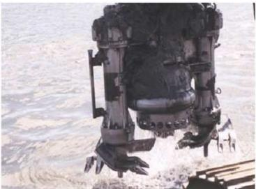
2. Its flow passage components is made of high-strength and wear-resistant alloy. It has large flow channel and is suitable for delivering pulp, coal slurry and sand etc. which contains relatively big solid particles.
