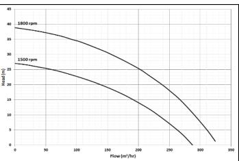
SKY 6" auto priming dewatering pump is the general purpose pump set. Designed for high volume and medium head. Excellent performance in Well-point dewatering, Sea Water transfer, sump pumping, Ground Water transfer and treated Sewer-by- pass.
